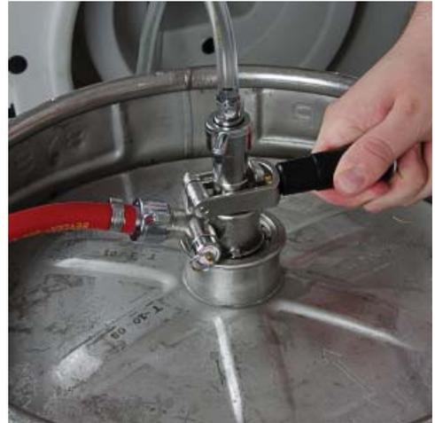
Bleed a small amount of pressure from inside the **KEG** by pulling the **BLEED VALVE** for 1-2 seconds.
