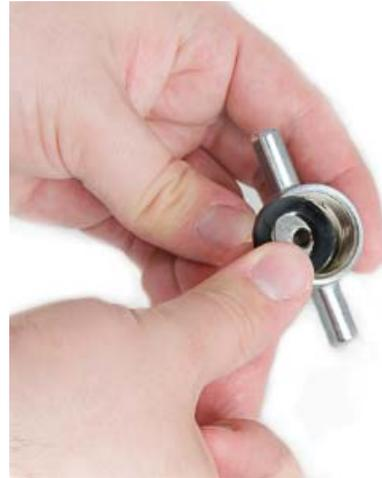
Hand-tighten the fitting onto the outlet on the SANKEY COUPLER until secure.
