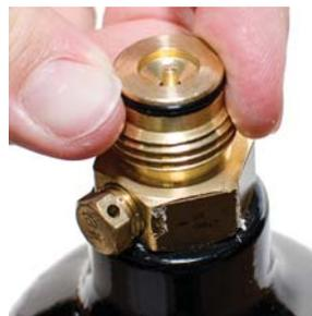
Slide new O-Ring into groove at top.
